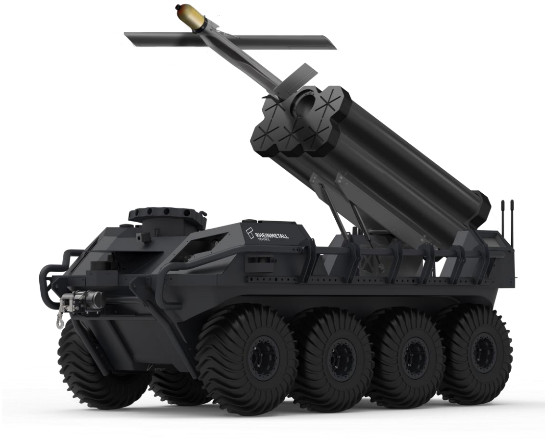
Rheinmetall Mission Master UGV armed with Warmate Micro Combat UAV from WB Electronics
