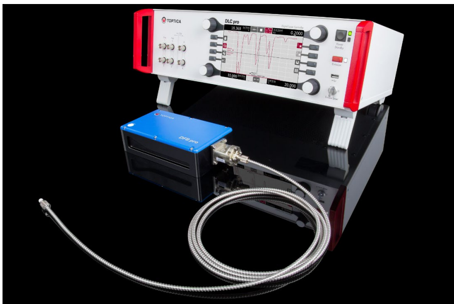
DFB pro 633 driven by DLC pro controller – mode-hop free tuning at 633nm
