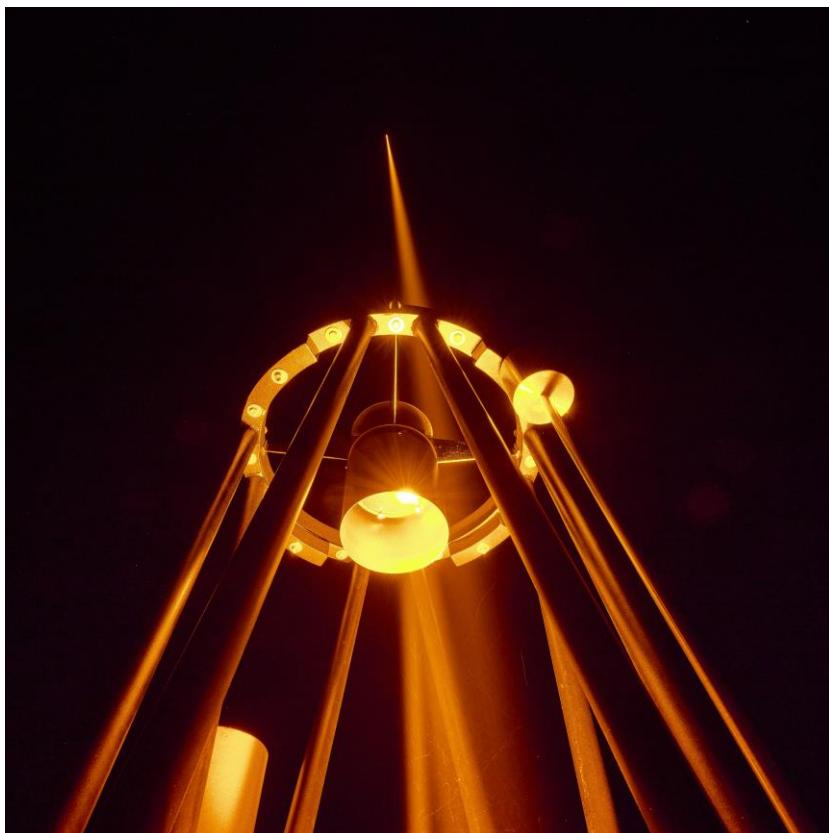
This image shows the CaNaPy laser equipped with TOPTICA Project's chirping system during the field test in Germany. The technology will be used to create artificial guide stars to measure how much the light is distorted by turbulence in the Earth's atmosphere. Correcting for the turbulence improves the sharpness of astronomical images significantly.
