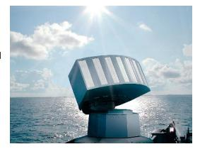
Ordinarily, MASS consists of between one and six trainable launchers. Each launcher can fire 32 Omni Trap special effect charges. Each launcher comes with a control unit and a data interface.
