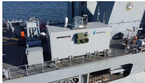
The ARGE's laser weapon demonstrator is integrated into a 20" container, installed on a previously integrated frame on the deck.
