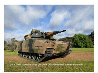
With the flexibility of the CRT fitted to the Lynx, the platform can be configured for a lighter all up weight (due to weight saving in track) to allow easier air transportation and to potentially reduce overall running costs through the service life of the vehicles.
