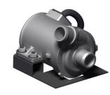
Electric coolant pumps make a significant contribution to emission control in modern engine designs. A flow rate that is not dependent on the speed of another drive enables demand-orientated cooling. This reduces the power requirement and at the same time lowers friction losses, fuel consumption and pollutant emissions. The pumps can be used in both electric and hybrid applications. They are characterised by their compact design and are available for different power levels from 50 to 2000 watts.
