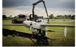
catapult, an optional net equipment for catching the drones when they land as well as equipment for rapid repair. The entire system is mounted on an HX truck with a swap body system made by Rheinmetall MAN Military Vehicles.
