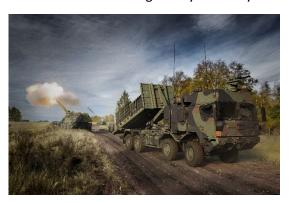
expanding the Bundeswehr's fleet of vehicles from the military HX family. The swap-body system's principal item of equipment is the hook-loader. Developed by Hiab, it can lift and set down swap-body platforms in the Bundeswehr inventory in virtually any type of terrain, with no need for additional cargo-handling equipment. As an alternative, the vehicles can carry a swap-body platform or a container via a standardized 20-foot ISO interface.
