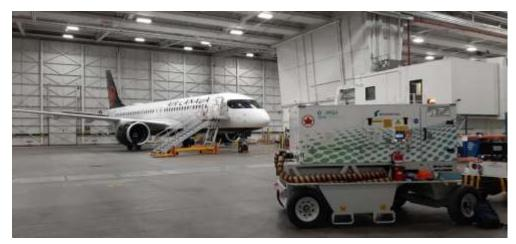
The eMSU provides pneumatic power to aircraft engines with its electrically driven turbine-type air compressor and embedded lithium-ion battery system that enable stand-alone operations, negating the need for external power, such as fixed power at the gate or a separate ground power unit. With its 250 ppm of air flow at 56 psia, sufficient to start the vast majority of aircraft engines, the eMSU is designed to start the engines of regional jets, narrow-body aircraft, and even wide-body aircraft.
