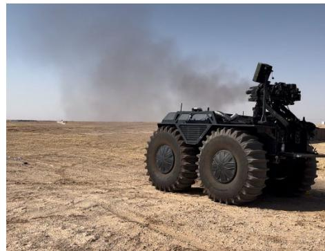
Designed as the last line of defence against small low-flying and fast-moving drones, Rheinmetall's ultra Short-Range Air Defence (SHORAD) system offers an engagement range from 50 to 800 m. The Mission Master XT uncrewed ground system (UGS) serves as the carrier platform.
