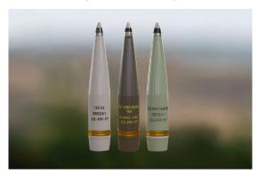
The ER02A1 high-explosive (HE) projectiles have a maximum range of 30 kilometres in the boat-tail (BT) variant and almost 40 kilometres in the base-bleed (BB) variant. The latter has a special device at the base of the projectile. This heats the air generated by the projectile itself in its trajectory, thus reducing drag and increasing the maximum range.
