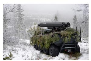
This only represents one of many possible configurations for the Mission Master SP – Fire Support. Featuring a fully modular architecture, this A-UGV can also be equipped with other weapon systems: 12.7mm calibre machine guns, a Dillon Aero M134D gun, or 40mm grenade launchers.
