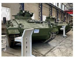
Rheinmetall acquired the overhauled 1A3 Marder IFV from the Bundeswehr. The company began overhauling the IFVs for immediate deployment at its own expense back in spring 2022. The corresponding work has since been underway at Rheinmetall's locations in Unterluess and Kassel.
