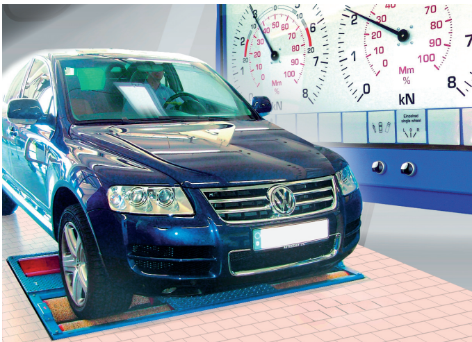
Typical test situation on MAHA test stand.
