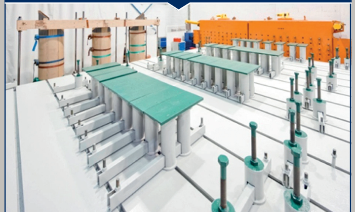
Core Stacking Platforms
