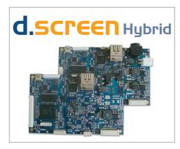
d.screen-Hybrid is a cost-effective innovative board solution for high performance USB 2.0 and/or Ethernet connected displays based on DisplayLink's latest DL1x5 device family and EliteSilicon's USB over IP technology.
