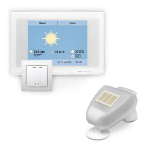
The WS1000 Style building control for a wide variety of ventilation scenarios, with control panel, WGTH-UP radio indoor sensor (central unit), and weather station
