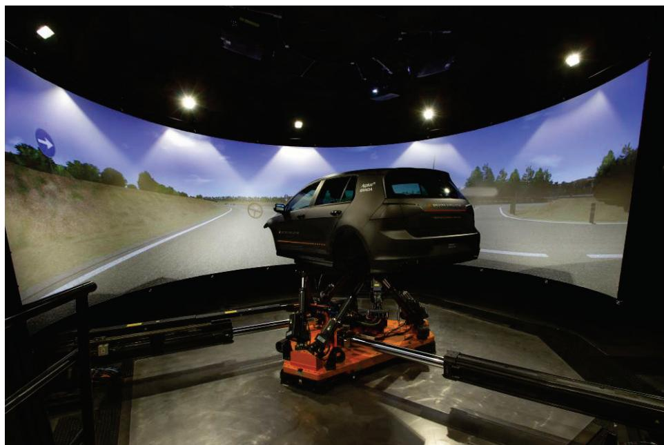
Applus+ IDIADA integrates virtual and physical testing with 2 new VI-grade driving simulators.
