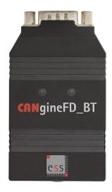
CANgineFD\_BT features a powerful 32-bit Cortex-M4 microcontroller clocked at 80 MHz that supports CAN FD data rates up to 10 Mbps. Together with the built-in Class 1 bluetooth module (100 m range), CANgineFD\_BT is the perfect low-cost solution to connect CAN and CAN FD networks with a smartphone or tablet.
