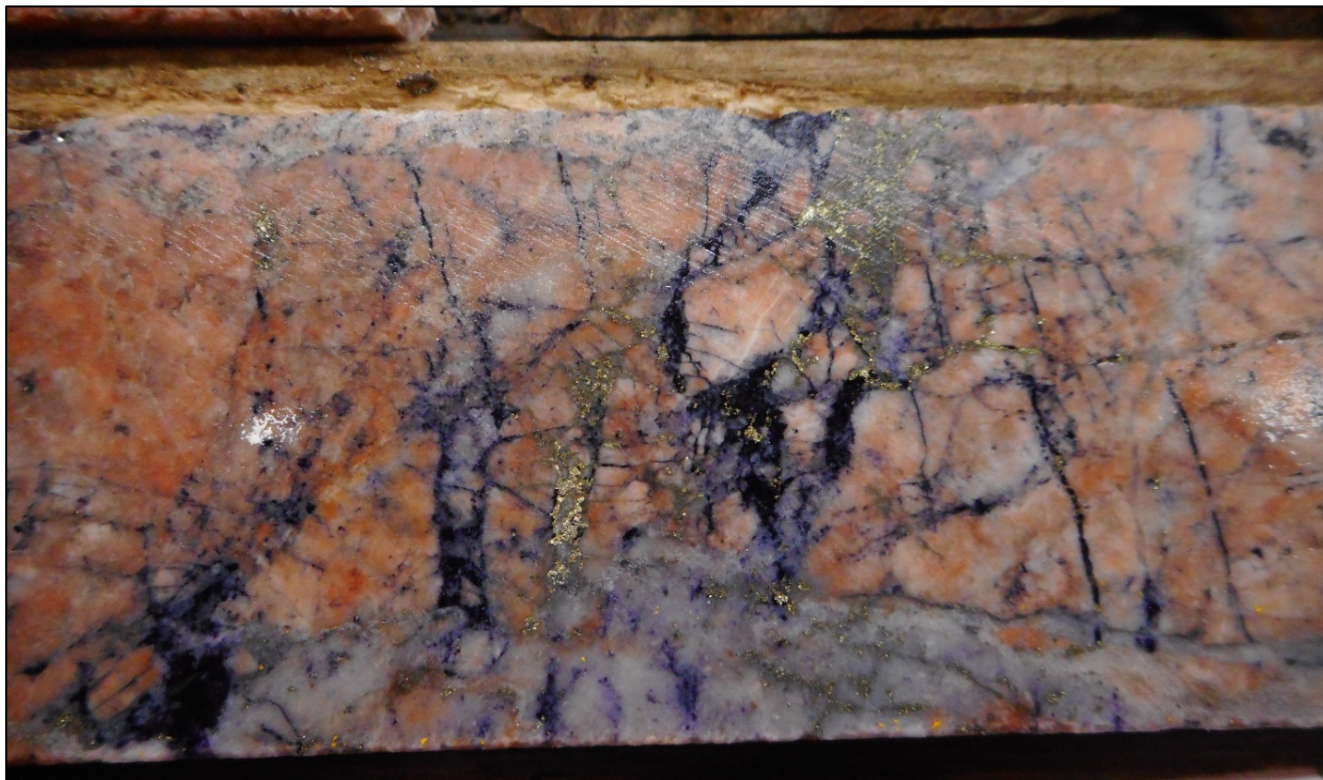
Fig. 4: Selected core from DO-20-281, from interval 152-153m, which graded 4.35 g/t Au. NQ core = 47.6mm diameter NQ core. Note that this core is not necessarily representative of all Douay mineralization.
