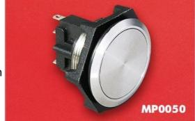
Rated at 5A, 250Vac, with single pole changeover, momentary switching the switch is designed with a minimum life expectancy of 1,000,000 mechanical operations and 35,000 electrical. The temperature rating is from -20 to +70°C and with front panel sealing to IP68 it is ideal for external applications.
