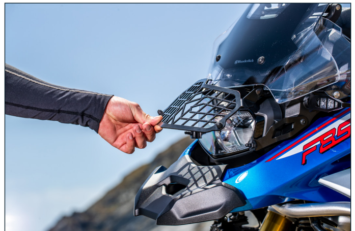
Protection grille variant made from high-quality stainless steel, powder coated; folded up permitted for road use
