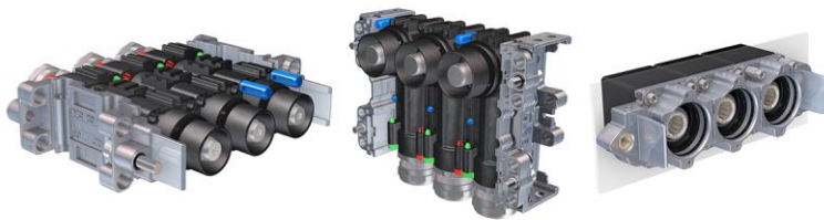
Fig. 2: The MPC in straight or right-angled versions, and as a receptacle, each with three modules. Up to five poles can be combined in a row, up to three rows can be stacked.
