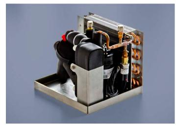
to the customer's liquid coolant circuit is a male R  $\frac{1}{4}$ " connector at the brazed plate heat exchanger and the system is suitable for a variety of coolant fluids. At 5°C water temperature and 200 W of cooling capacity its power consumption is only 115 W.
