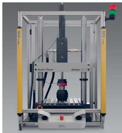
Servo-hydraulic testing machine Amsler HC 5 for testing rubber mountings
