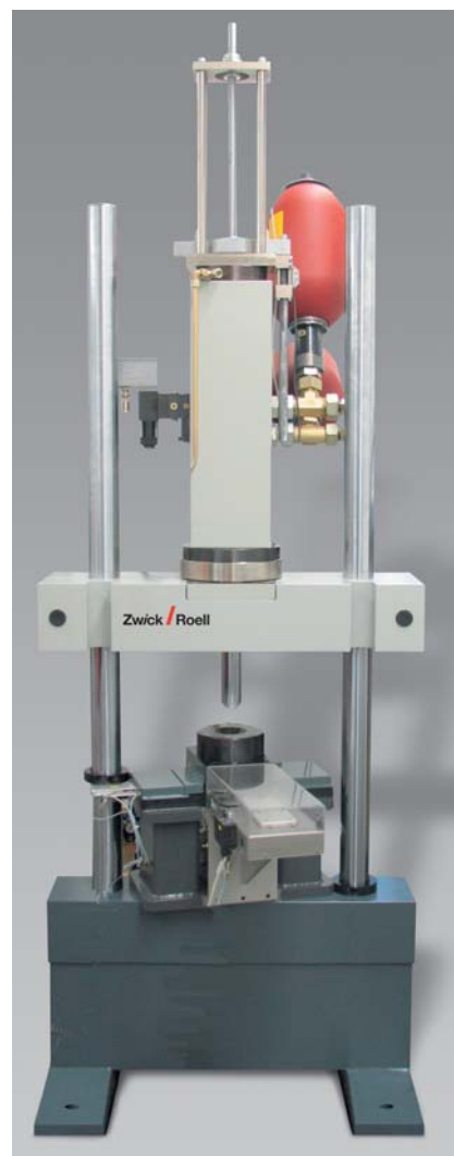
High-speed testing machine equipped for multiaxial impact tests
