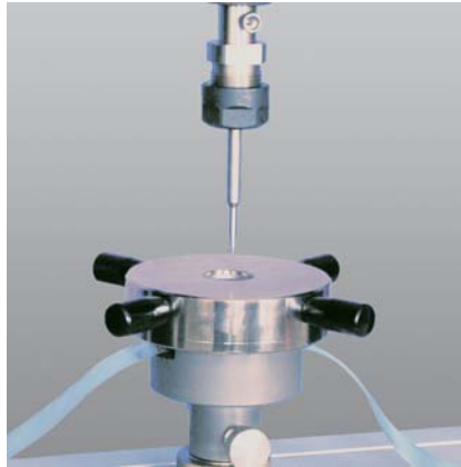
Puncture test device acc. to EN 14477
