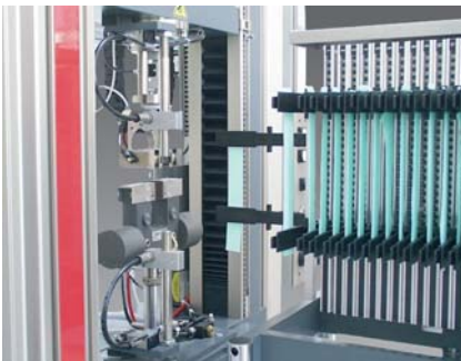
“roboTest F” is perfect for testing flexible specimens, i.e. plastic film.
