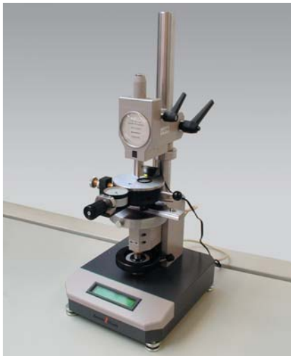
IRHD Micro Compact hardness tester 3103
