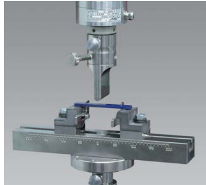
Flexure tool according to ISO 178
