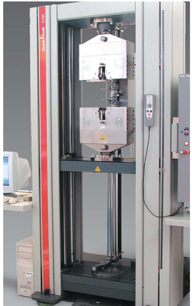
Allround-Line Z100 equipped with pneumatic grips and Macro extensometer
