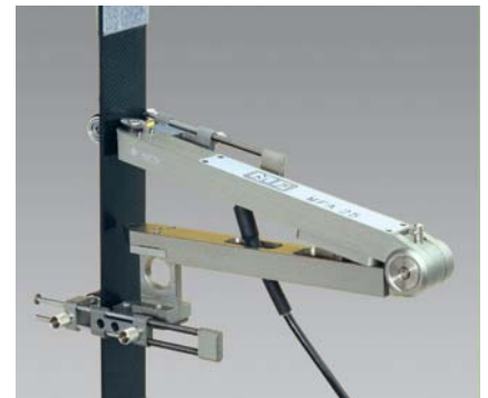
Analogue clip-on extensometer
