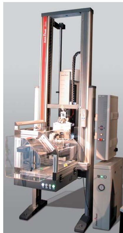
The “roboTest B” tester can switch from tensile to flexural tests.
