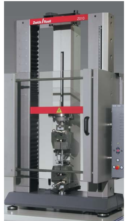
Materials testing: Tensile test according to ISO 527-2
