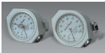
Analog Shore A and D hardness tester: Hand-held devices
