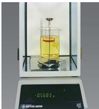
Digital balance and kit for the determination of density, gravimetric method, (4106.69)
