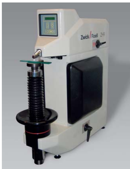
Rockwell hardness tester for scales R, L, M, E, K and \alpha
