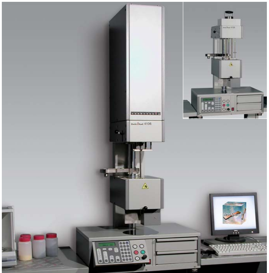
Extrusion plastometer Zwick 4106.200 with automatic weight change unit. Upper right: the basic version with manual weights.
