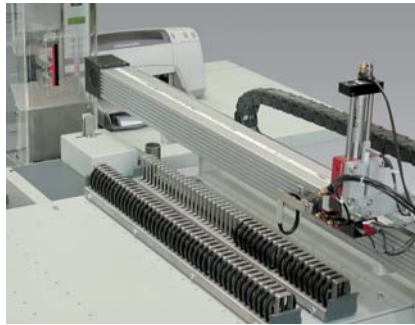
Variant of “roboTest L” for testing of ring-type rubber specimen
