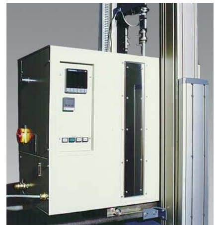
The controller and the opening for extensometers on the rear left side
