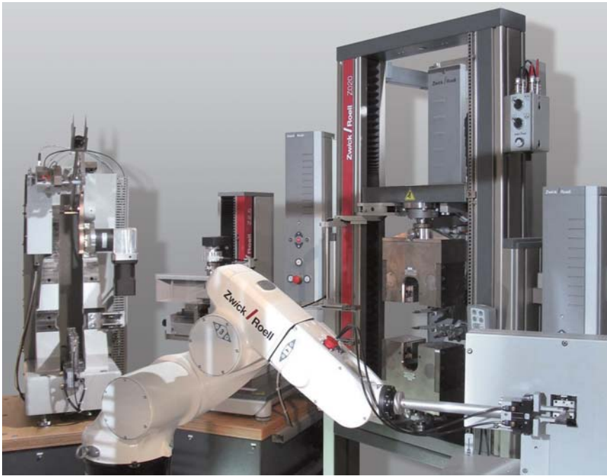
“roboTest R”: The illustrated system integrates tensile, flexural, and Izod testing.
