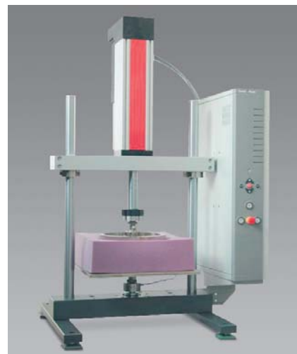
This machine can be used for constant load pounding tests as well as for static compression and indentation hardness
