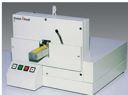
Automatic cross-section measuring device (Ref. 066998.00.00)
