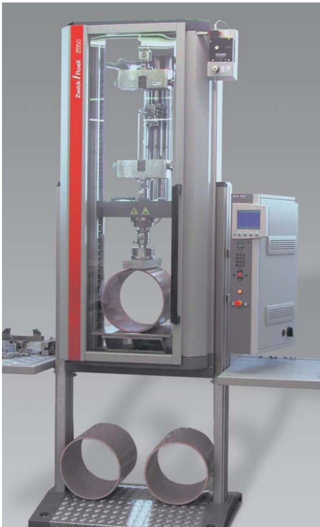
Allround-Line Z050 in an extended version for testing tensile characteristics and ring stiffness on plastic pipes
