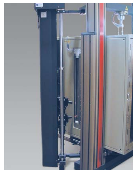
Optical extension measurement in a temperature chamber
