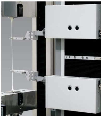
The multiXtens-extensometer combines high-resolution and long-stroke measurement
