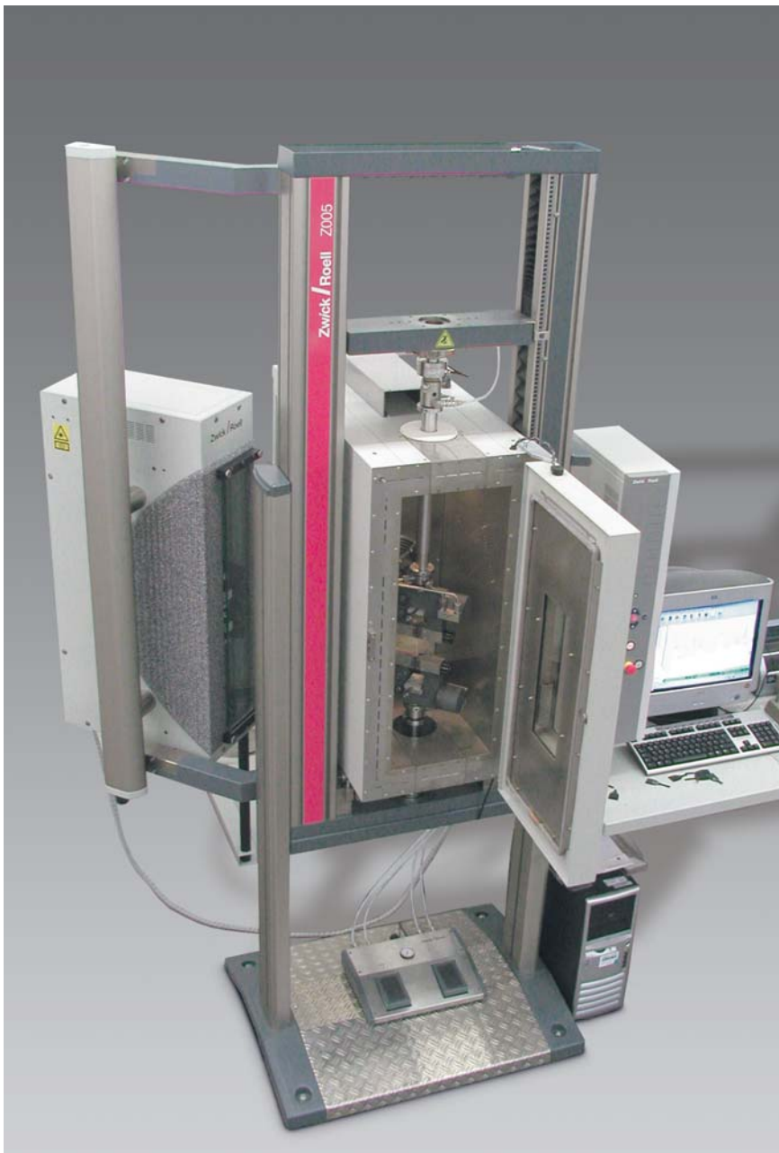
Temperature chamber, optiXtens extensometer and pneumatic grips mounted in a material testing machine Z005
