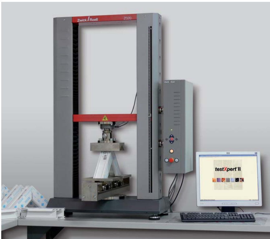
Components testing with ProLine: Determination of the stiffness of window frames
