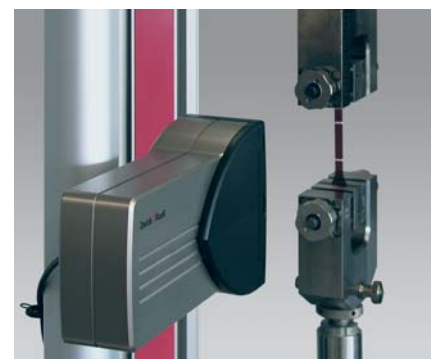
The videoXtens is adapted to the test by selecting suitable field of view
