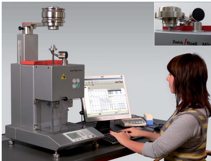
Modular plastometer Mflow for comfortable MFR and MVR measurements. Here shown with optional separation shield, piston travel transducer, automatic weight release system and PC software control.
