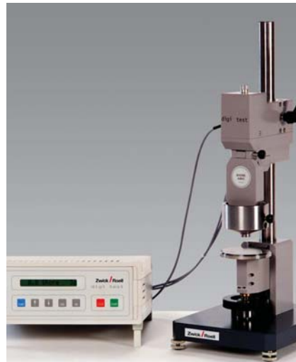
IHRD/Shore hardness tester 3105 digi test
