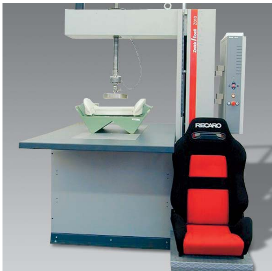
The C-frame is used for compression and indentation hardness tests of large foam parts
