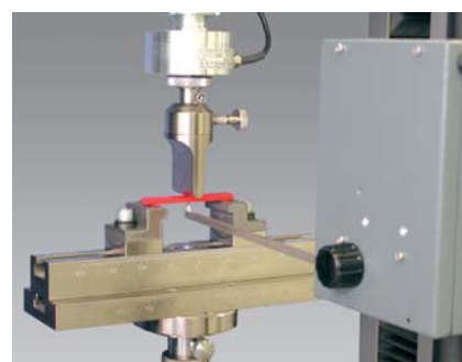
The 3-point flexure transducer has been developed particularly for this test
