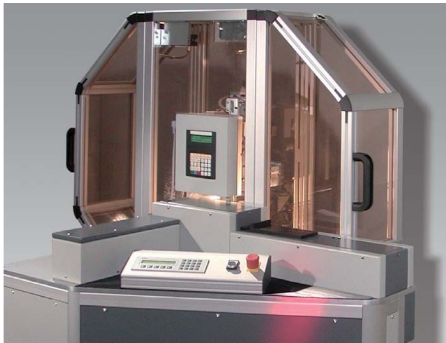
“roboTest I”: Charpy impact testing with a large temperature range.
