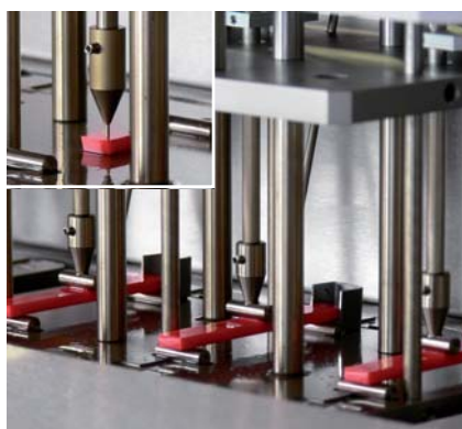
Upper: Vicat softening temperature, VST, Lower: HDT, heat deflection temperature.
