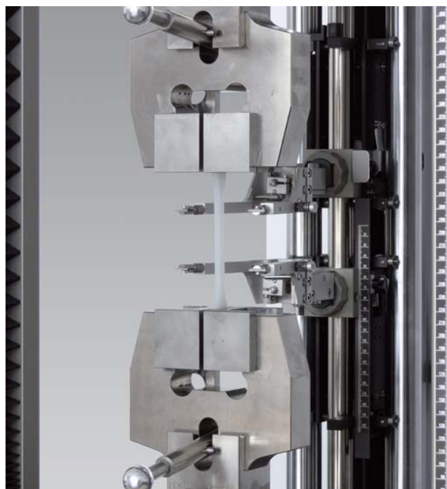
The mechanical long-travel-extensometer is designed for measurements on rubber and plastics.
