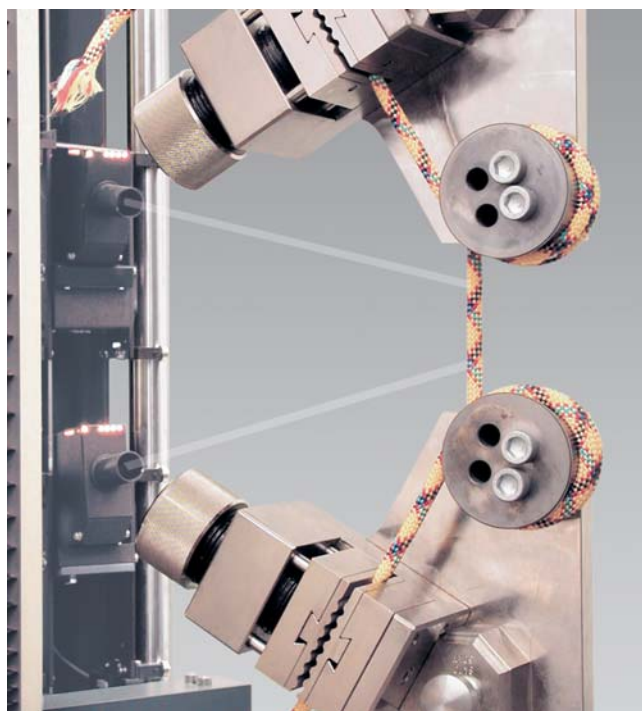
The optical long-travel-extensometer allows a contact-free measurement of the specimen marks attached on the specimen
