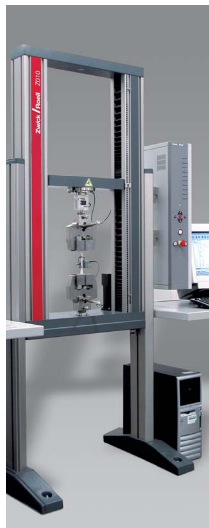
Alround-Line Z010 equipped for tensile testing
