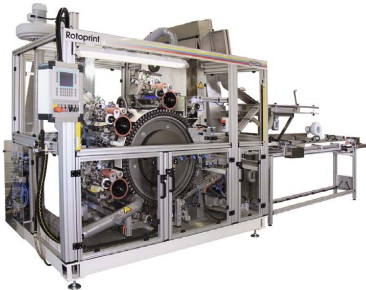
Illustration 2: „Rotoprint“ – Fully automated system for plastic bottle caps – Rotary tampon printing
