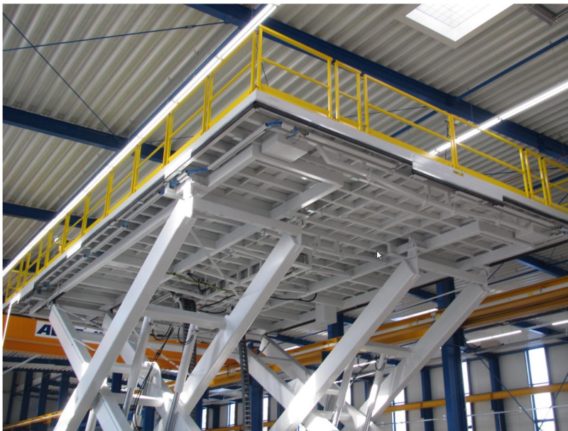
Fig. Nr. 11 & 12: Foto and 3D model with scissor lift work platform at test cell
