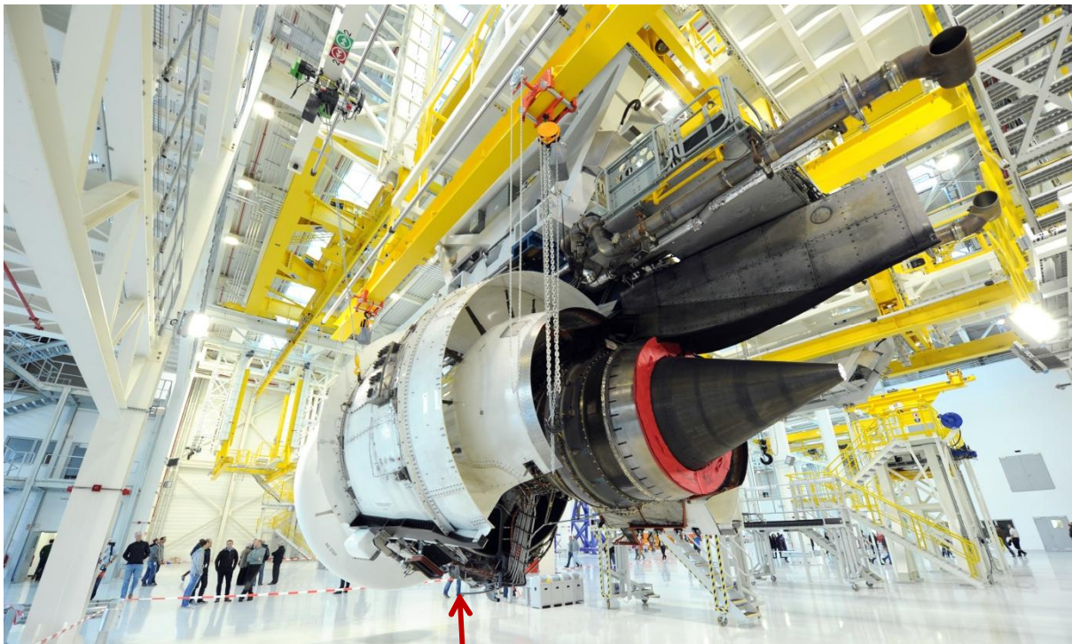
Fig. Nr. 1: TRENТ XWB Engine on one of four CTI Systems VHWS
