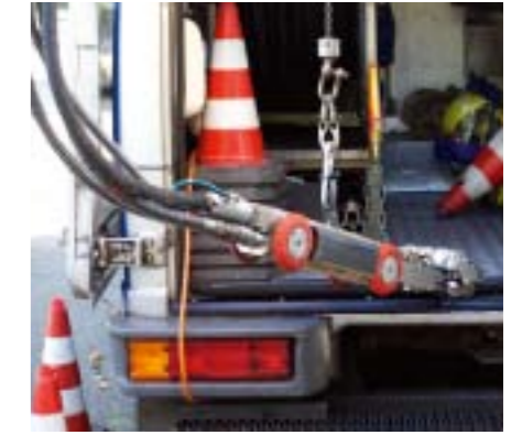
» High-tech in action. The Berlin water operations use remote controlled robots to inspect the narrowest channels.
