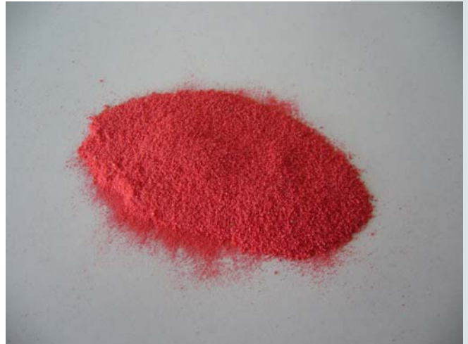
Picture 5: Analysis fineness after milling with the PULVERISETTE 14, sieve 0.5mm
