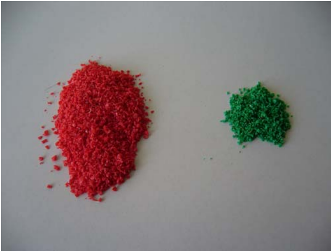
Picture 4: Pre-grinding with PULVERISETTE 19, sieve 2mm
