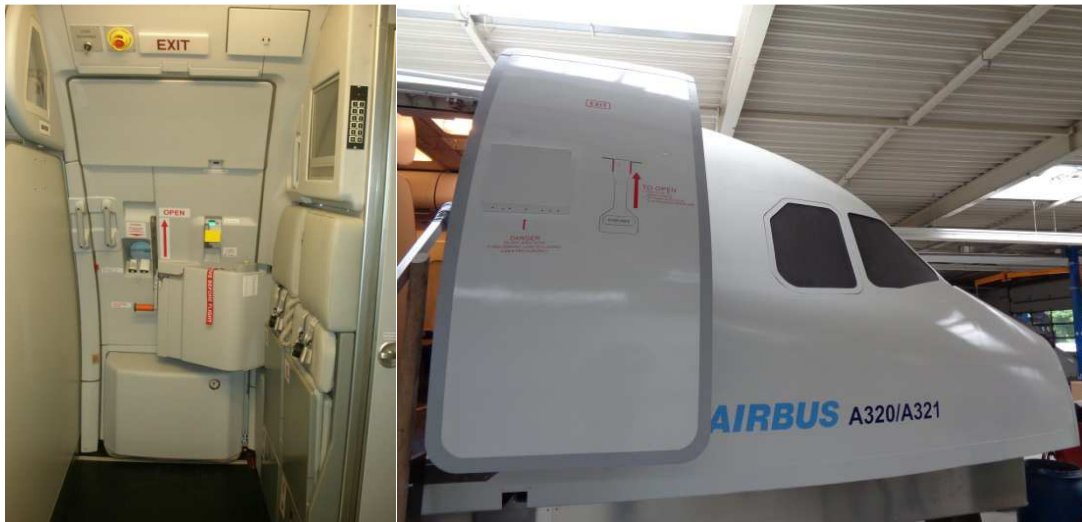
Fig. 2: The door trainer simulates conditions such as door blockages, fire and other hazards that occur during emergency situations, such as hard landings or crashes
