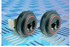
The PX0839/PC is designed for direct PCB mounting. The connector is rear-of panel mounting, which in addition to providing an anchor point for the PCB,
