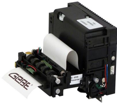
**Protects Print Mechanism and saves repair cost: GeBE-COMPACT Plus Printer with Presenter Unit**
