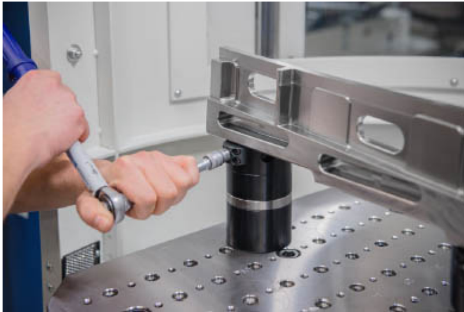
Bild Nr. 99-05 AM_KO-Lösen.jpg. Minimize set-up times with AMF zero-point clamping technology: the workpiece is clamped in just a few simple steps.
