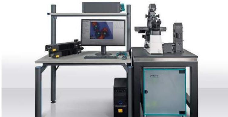
Top: Confocal Raman microscopy - alpha300 Ri for inverted Raman microscopy
