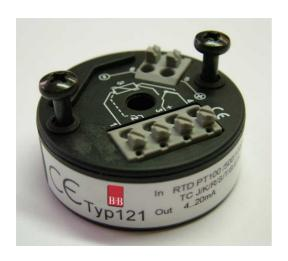
The digital Transmitter type 121 for DIN B connection head mounting is a programmable transducer for different resistance sensors and thermocouples. It converts the measured value into a proportional analog signal 4 to 20 mA. The current output – temperature linearity is better than 0,1%.
