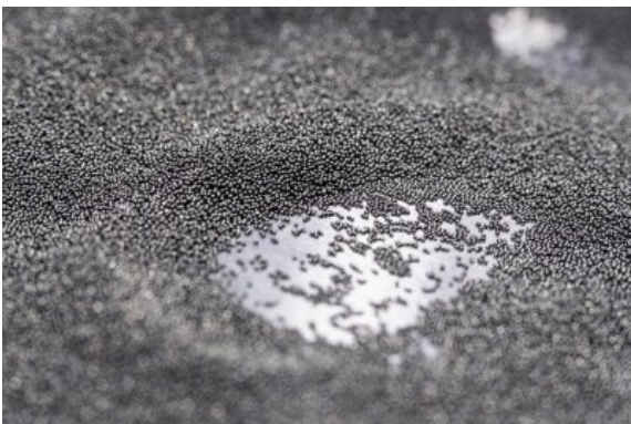
Picture 1 - Shot (steel balls) for surface compaction.
