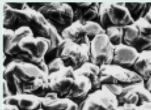
ohne Additive, j = 140 \text{ A/dm}^2 , v = 70 \text{ m/min}
