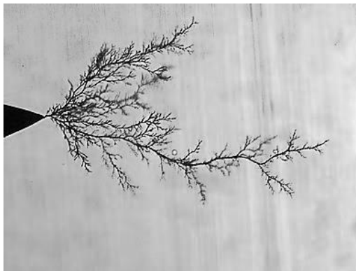
Formation of a conductive path on or in insulation materials (Source: CMC)
