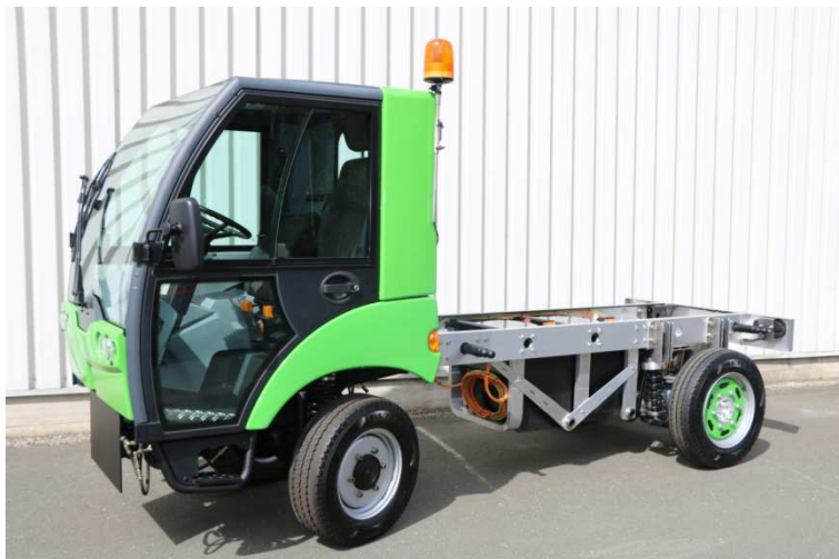
Fig. 1: Baumüller has developed a compact drive system with a very high level of energy efficiency for a fully electric municipal vehicle. The vehicle is designed in series production for a speed of up to 80 km/h and has a range of 100 kilometers
