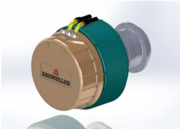
Fig. 2: The electric axle developed by Baumüller as a drive system is in duplicate on the rear axle or 4-fold with all-wheel drive. It consists of a Baumüller DSA synchronous external rotor motor with planetary gear and integrated line electronics with motor controller and converter
