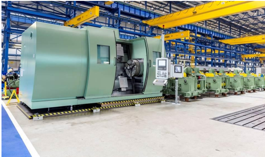
Type TCG threading machine with rotating pipe supplied by SMS group to JFE Chita Works.
