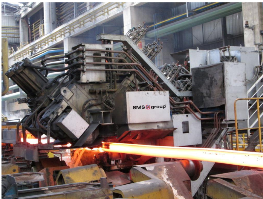
EBROS system in operation. Shown is the welding stage.
