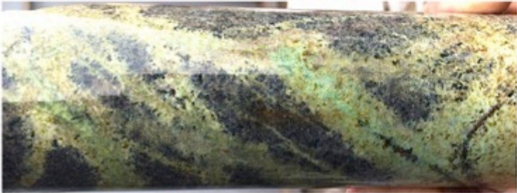
Figure 6: Illustrates copper oxide endoskarn mineralization within the Ccasccabamba diorite sill.
