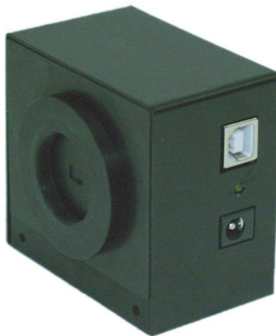
PhasePro camera shown actual size. 70 x 64 x 45 mm (W x H x D) C-mount threaded mounting flange
