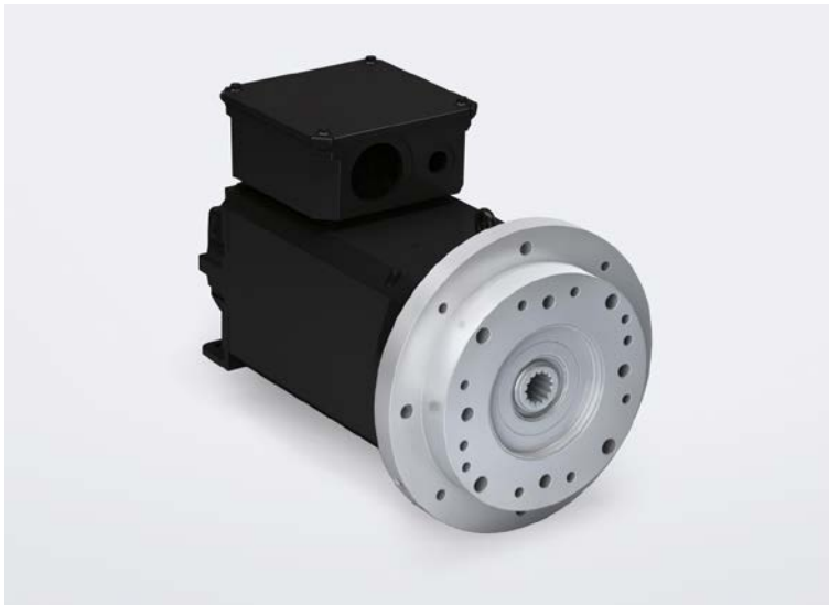
Figure 2: The new alternative interface with internal splines eliminates expensive transmission elements, such as couplings and pump supports. This option is available for servo motor series DS2, DSP, DSD2, and DSC. It saves costs and optimizes installation space
