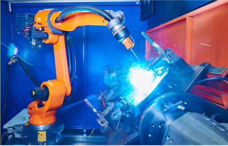
Fig. 1: Qirox QRH-280 in action: From special technology modules via the box PC and the control technology to the drives. In addition to the motors, Baumüller has also taken over the complete automation for the Cloos robot
