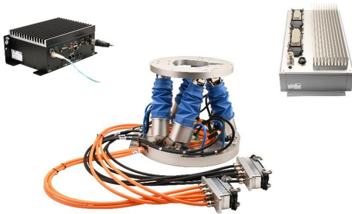
The positioning system developed by Physik Instrumente (PI) for the LuFo VI-1: ADMAS research project consists of a controller (left), a hexapod (center), and the driver electronics (right). The controller and driver communicate via fiber optic data transmission. The hexapod and driver are IP54 sealed to protect against CFK dust, coolants, and lubricants. (Photo: Physik Instrumente (PI))
