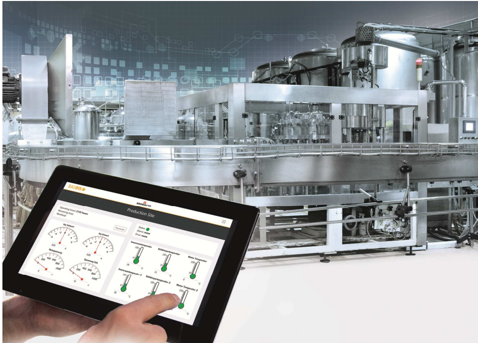
Figure 1: With BAUDIS IoT, machines and systems can be monitored and analyzed remotely or locally, thereby reducing unexpected downtimes and identifying potential for process optimization
