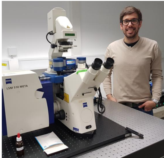
Dr Henri Franquelim and the newest JPK NanoWizard® ULTRA Speed AFM mounted on top of a Zeiss LSM 510 META confocal microscope
