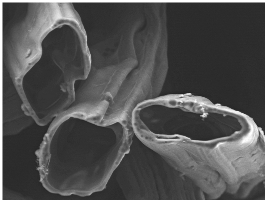
Greatly enlarged image of a cross-section of regenerated cellulose fibres. ©Kelheim Fibres
